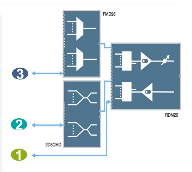
Start with direct connect channels and expand with external multiplexers as traffic growth is confirmed
